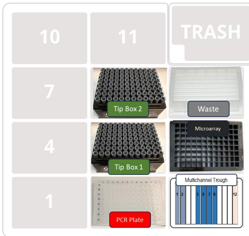
Figure 2. Labware Arrangement on the Opentrons OT-2 Deck
