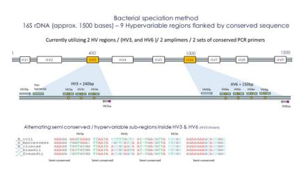
regions known to contain sequence changes that are species specific (well-known rDNA hypervariable domains). Pathogen Dx has demonstrated that a single multiplex PCR reaction that is targeted to HV3 and HV6 (in 16S) and an analogous HV region in 28S (for fungi) can generate amplicons which can be used to 'Detect and Discriminate' individual
