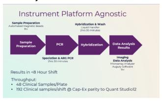
Sample preparation to results in a single shift. D³ Array-UTI is instrument platform agnostic enabling easy integration into the existing molecular testing laboratories and creating flexibility for laboratories new to molecular testing. Any of the many established sample preparation methodologies can be used, the most common being automated magnetic bead-based systems. Sample processing typically takes approximately one hour. Purified DNA is amplified using any standard
